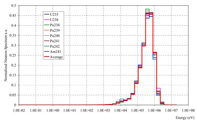
Figure 12. 33 energy groups delayed spectra and average delayed spectrum
