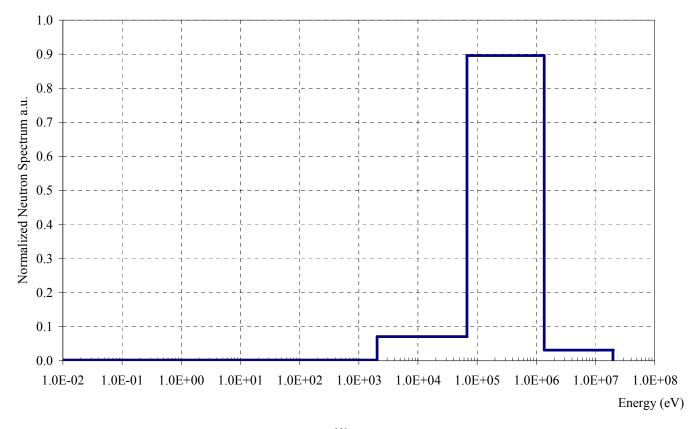
Figure 10. 4 energy groups <sup>239</sup>Pu delayed spectrum
