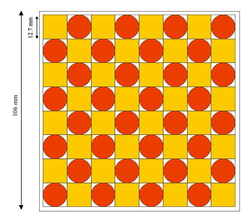
Figure 2. XY loading of the MUSE-4 U/Pu MOX fuel subassembly
