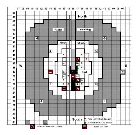
Figure 5. XY view of the MUSE-4 SC0 1086 fuel cells configuration
