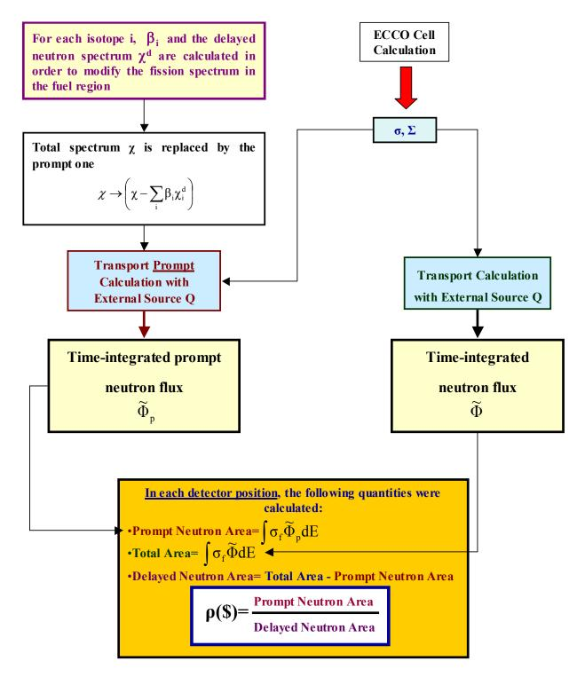
Figure 9. Flow chart of the assessed ERANOS calculation procedure simulating the PNS area method
