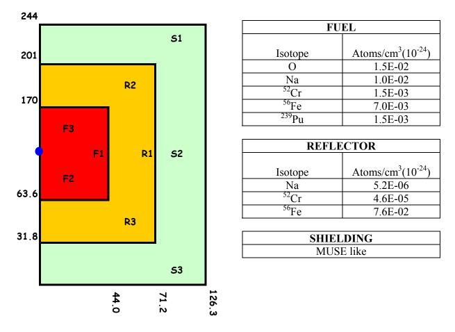
Figure 1. RZ simplified configuration for tests
