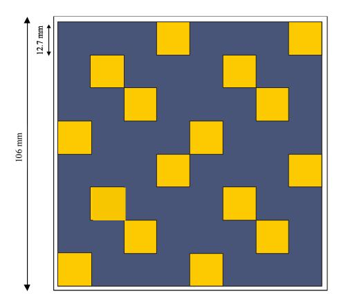
Figure 3. XY loading of the MUSE-4 sodium and stainless steel reflector subassembly
