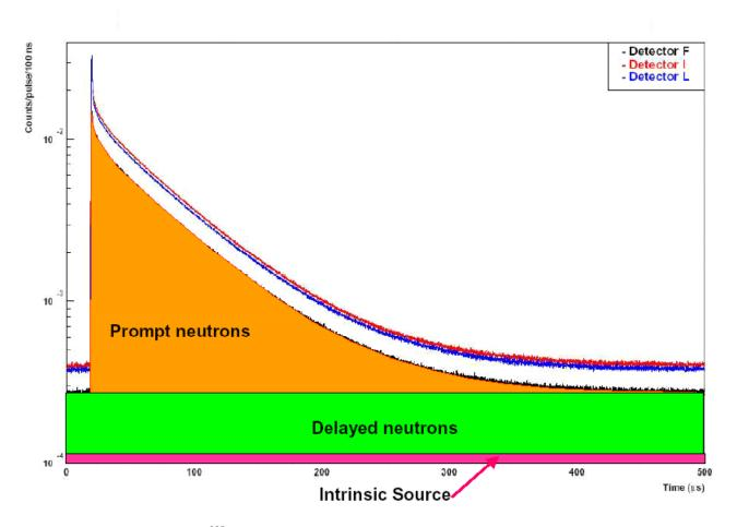
Figure 8. <sup>235</sup>U detector response to a D-T external neutron pulse
