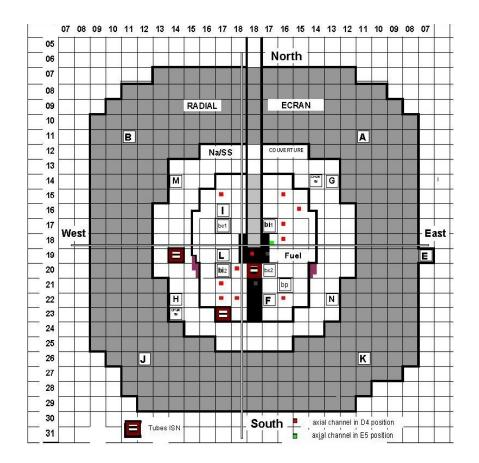
Figure 4. XY view of the MUSE-4 SC0 1108 fuel cells configuration and <sup>235</sup>U detectors position
