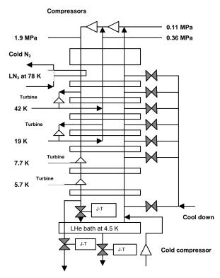
Figure 4.8 Typical helium cryogenic plant process for ITER [38]
