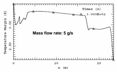
Figure 6.14 Temperature margin along the length of the TF feeder (With 5.0 g/s helium mass flow rate)
