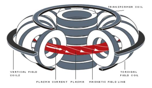
Figure 4.1 Tokamak principle
