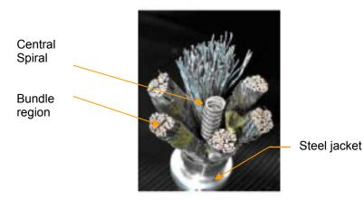
Figure 6.1 Cross-sectional view of dual channel CICC for the ITER LTS feeder
