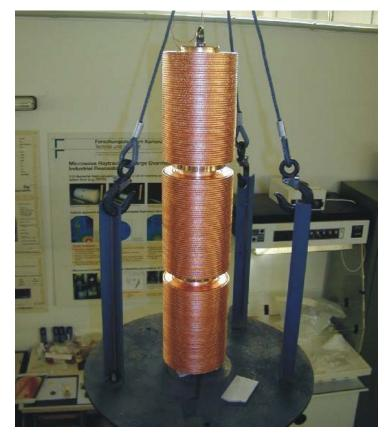
Figure 8.15 Photograph of the conventional heat exchanger of the 70 kA HTS current lead [63]
