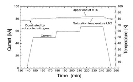
Figure 5.8 HTS CL operations at 68 KA with atmospheric LN<sub>2</sub> cooling [68]
