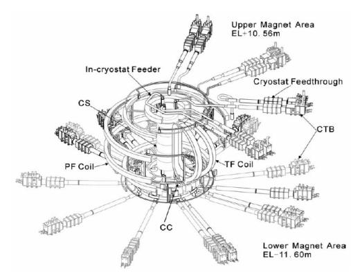
Figure 4.5 An elevation view of the magnets and feeders in ITER [2]
