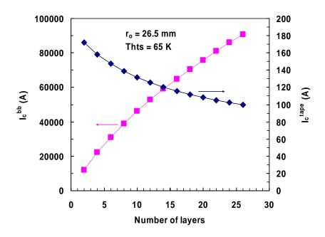
Figure 8.8 Critical currents of the feeder and the tape at 65 K as a function of the number of Bi-2223 layers wound onto a flexible stainless steel pipe of 26.5 mm outer radius
