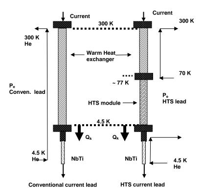
Figure 5.1 Working principles of conventional and HTS current leads
