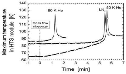
Figure 5.9 LOFA tests of 70 kA HTS CL with helium and LN<sub>2</sub> cooling [69, 70]
