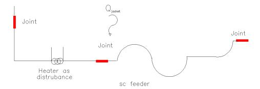
Figure 6.15 Simulation of a conductor disturbance by means of an external heater
