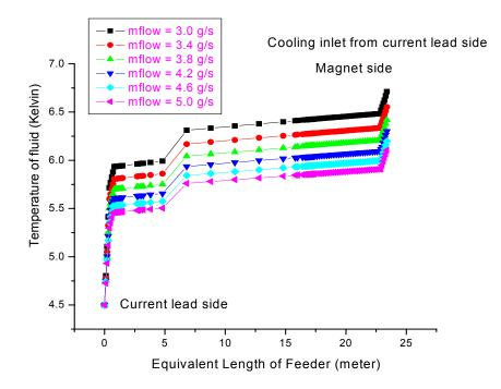
Figure 6.10 Temperature profile of the TF feeder for different helium mass flow rates
