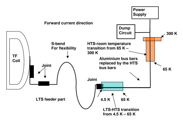
Figure 8.1 Conceptual layout of the TF current feeder system with a combined LTS / HTS bus bar system in case of 50 K helium cooling
