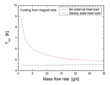
Figure 6.11 (b) Temperature at the outlet with mass flow rates
