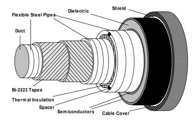
Figure 8.2 Illustration of a single-phase warm dielectric power transmission cable [84]
