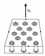
Figure 2.3 The mixed state in Type II superconductors
