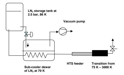
Figure 8.16 Sub-cooled LN<sub>2</sub> cooling for the HTS bus bar and its transition at 75 K [93]
