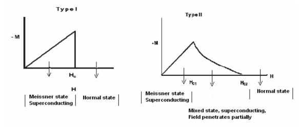
Figure 2.2 The schematic magnetization behaviour of the Type II superconductors [14]
