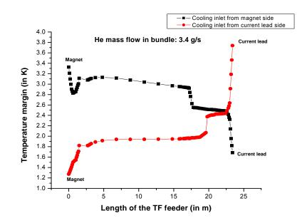
Figure 6.11 (a) Cooling modes comparison study for the TF feeder
