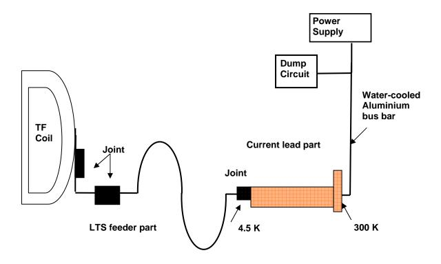
Figure 1.1 Schematic layout of the present design of current feeder system for ITER
