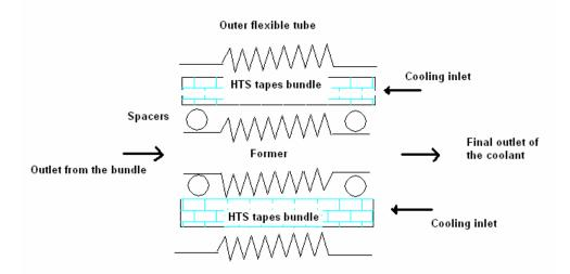
Figure 8.14 Cooling scheme of the HTS feeders for ITER
