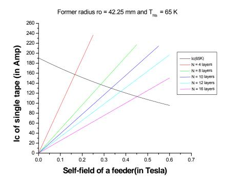
Figure 8.7 Determination of the critical current of Bi-2223 tapes in the multilayer feeder at 65 K.
