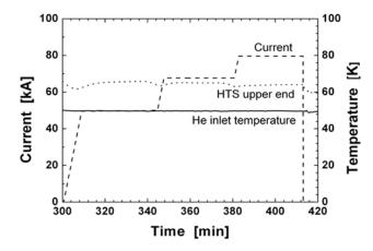
Figure 5.6 HTS CL operation with T<sub>He,in</sub>=50 K. The temperature of the HTS module upper end was at approx. 65K [68]
