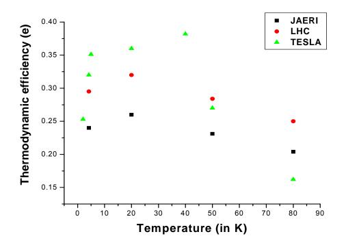
Figure 3.2 Temperature versus thermodynamic efficiency of the helium plant
