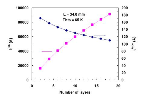
Figure 8.9 Critical currents of the feeder and the tape at 65 K as a function of the number of Bi-2223 layers wound onto a flexible stainless steel pipe of 34.0 mm outer radius
