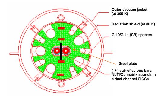
Figure 6.2 Cross-sectional view of a LTS feeder for ITER
