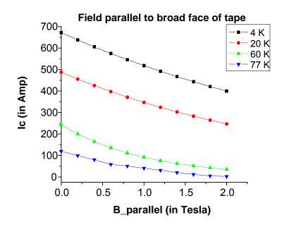
Figure 8.5 Critical current characteristics of a single Bi-2223/Ag/AgMg tape
