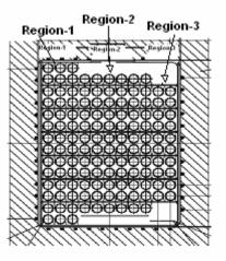
Figure 6.4 Cross-sectional view of the TF winding pack
