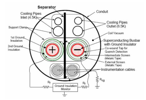
Figure 4.7 Cross-section of the In-cryostat feed through with cooling piping and instrumentation cables (courtesy from ITER DDD report [2])
