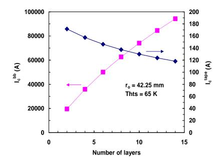
Figure 8.10 Critical currents of the feeder and the tape at 65 K as a function of the number of Bi-2223 layers wound onto a flexible stainless steel pipe of 42.25 mm outer radius
