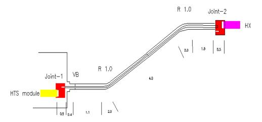
Figure 8.17 Model of an HTS bus bar with two bends
