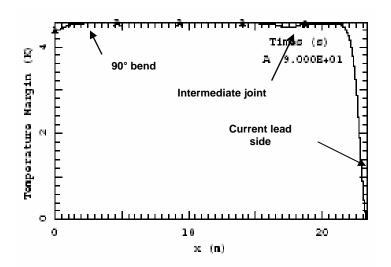
Figure 6.18 LOFA event followed by a magnet dump with steady state heat load
