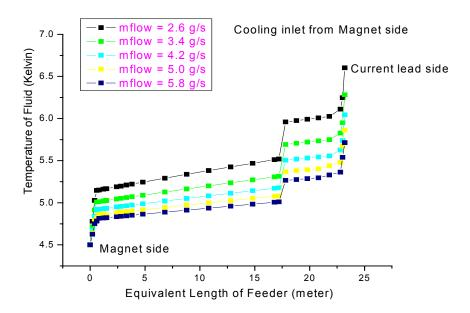
Figure 6.9 Temperature profile of the TF feeder for different helium mass flow rate
