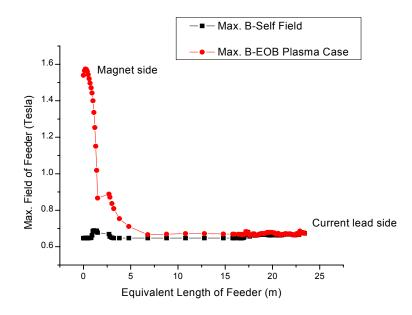
Figure 6.6 Comparison of the magnetic field profile along the TF feeder
