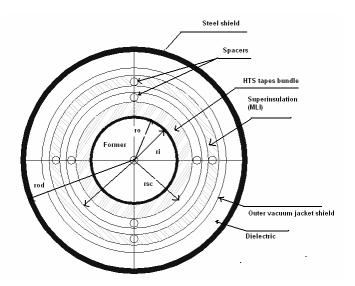
Figure 8.3 Cross-section of an HTS power cable showing the main dimensions
