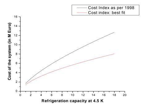
Figure 4.9 Cost estimates for several kW helium refrigeration systems
