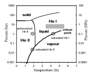
Figure 3.3 Phase diagram of helium (P-T diagram) [31]
