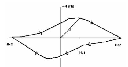
Figure 2.4 Magnetization – field characteristics in Type-III superconductors [16, 17]
