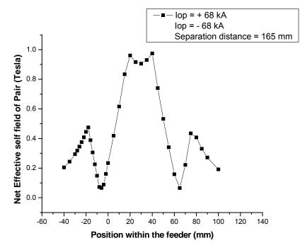
Figure 6.7 Self-field and stray field of a (+/-) pair of feeders at 68 kA
