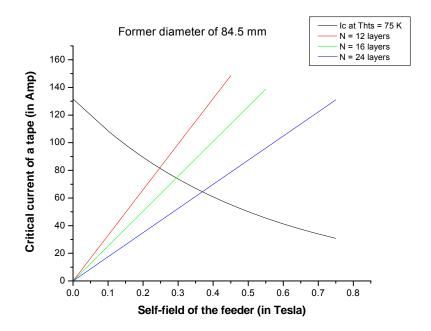
Figure 8.11 Determination of the critical current of Bi-2223 tapes in multilayer feeder at 75 K.
