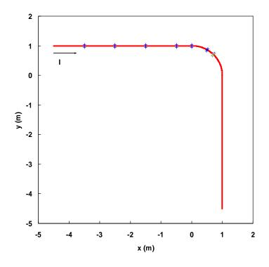
Figure 8.13 Conductor arrangement used for the estimation of the magnetic field at the positions marked by the crosses.
