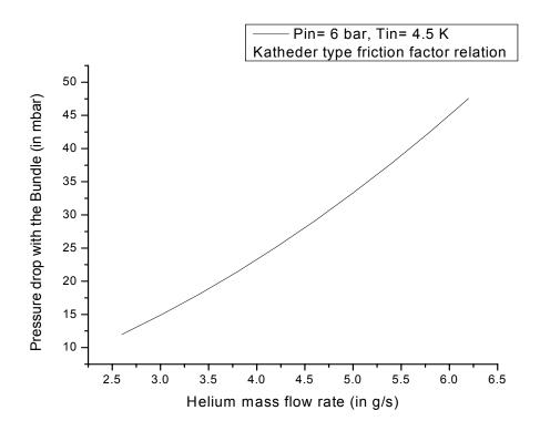
Figure 6.8 Pressure drop vs. mass flow rate characteristic for the TF feeder
