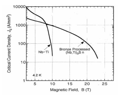
Figure 2.7 Non-Cu J<sub>c</sub> (4.2 K) vs B curves for LTSs [18]
