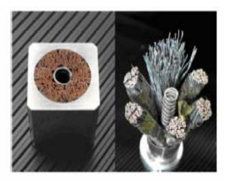
Figure 4.4 Cross-sectional view of the CSMC conductor (left) and TFMC conductor (right)
