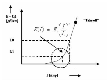
Figure 2.5 E – I characteristics for technical superconductors [16]
