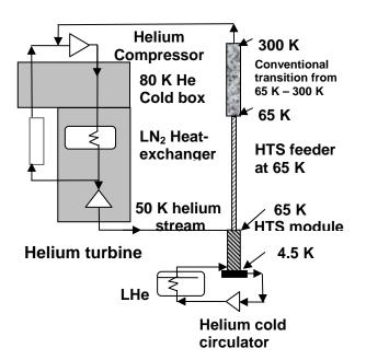
Figure 8.15 50 K helium cooling scheme for the HTS feeder system [93]
