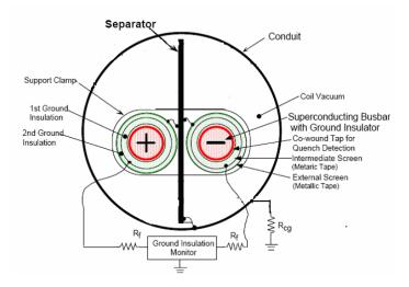
Figure 6.3 Double insulation scheme and ground insulator monitor for a (+/-) pair of sc bus bars
