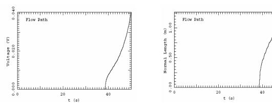
Figure 6.17 (a) Voltage develops only at 38 s
