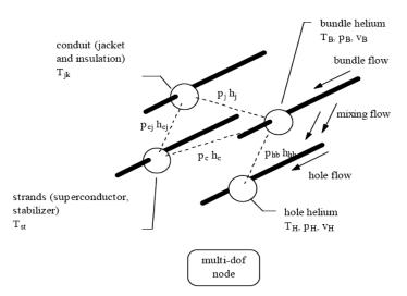
Figure 6.12 Basic finite element used in Gandalf, showing the degrees of freedom and the coupling of the thermal and flow components
