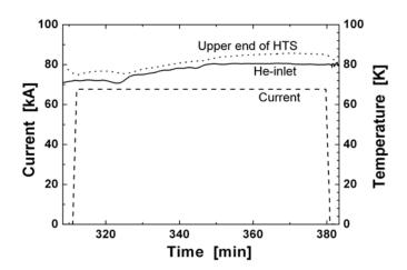
Figure 5.7 HTS CL operation at 68 kA with T<sub>He,in</sub>=80 K. The temperature of the HTS module upper end was at approx. 85 K [68].
