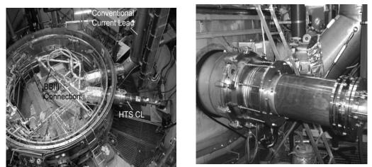
Figure 5.4 HTS CL installation in the TOSKA Figure 5.5 Horizontal installation of HTS CL
