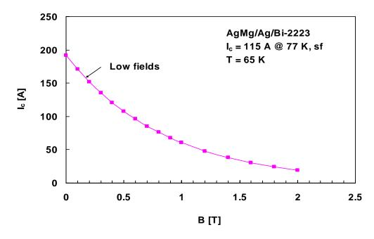
Figure 8.6 Critical current of Bi-2223/Ag/AgMg tapes as a function of the magnetic field applied along the broad face of the tapes at 65 K
