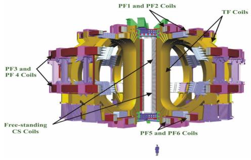
Figure 4.3 A 3-D view of the ITER main magnet system
