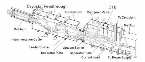
Figure 4.6 Cryostat feed through and CTB with valves and current leads [2]
