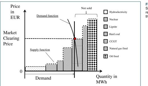
**Figure 11** Schematic representation of the Merit Order<sup>162</sup>
