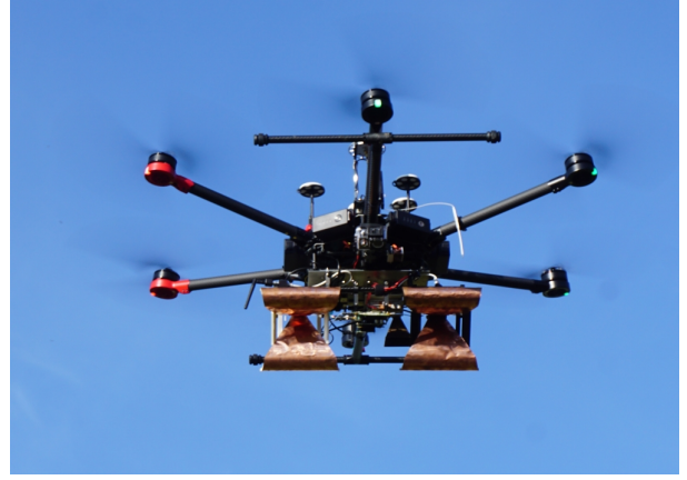
Fig. 8. Photo of the carrier platform DJI M600 Pro equipped with two TEM-horn antennas.
