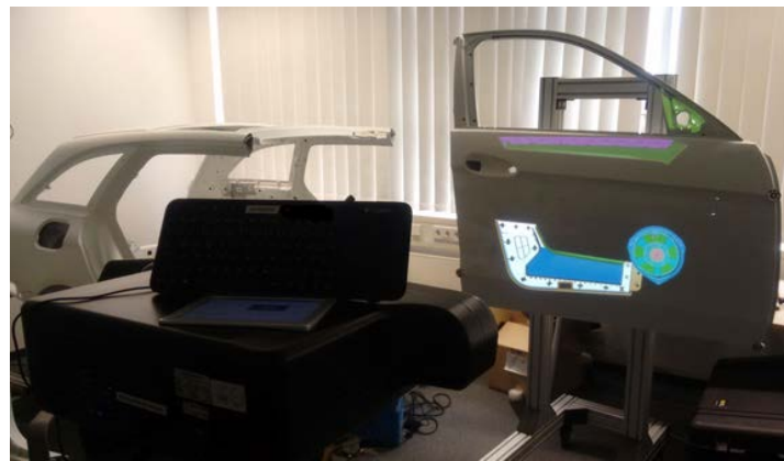
Figure 9.7: Visual assembly support using video-based projective SAR to display assembly parts on a door
