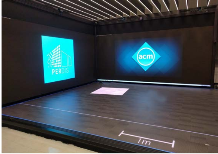
Figure 8.12: The VMS apparatus consists of two 16 sqm, L-arranged LED walls next to a 54 sqm large-scale LED floor [239, 245]
