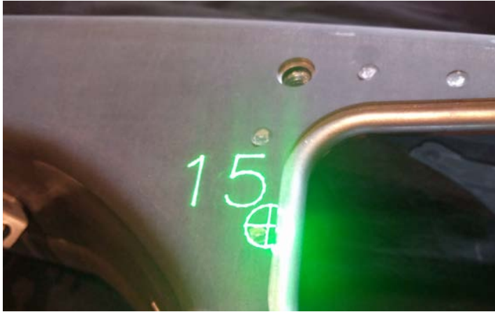
Figure 9.5: PMU quality inspection check by laser-based projective SAR to display potential offsets between DMU and PMU
