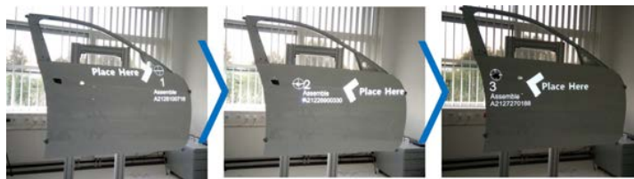
Figure 9.9: Alphanumeric assembly task information on generic PMUs using video-based projective SAR
