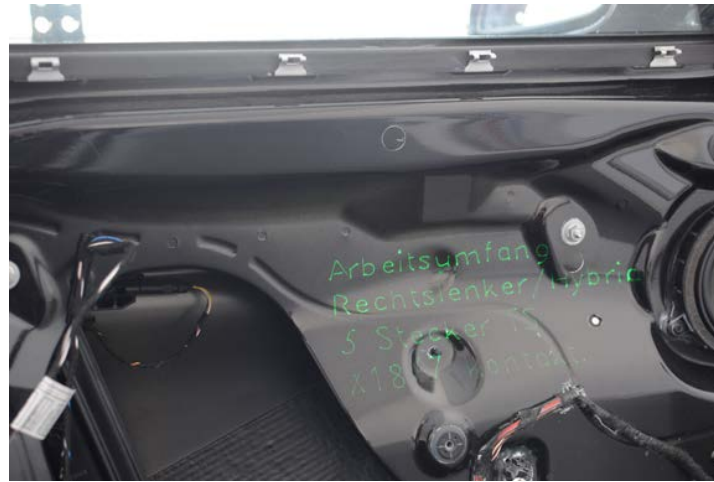
Figure 9.10: Alphanumeric assembly task information on generic PMUs using laser-based projective SAR
