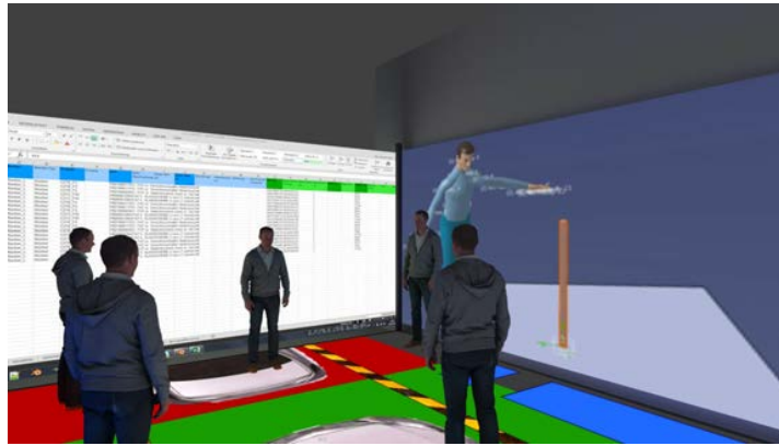
Figure 5.6: Rendering of large multiple wall-sized large high-resolution visualization devices with a LED floor.
