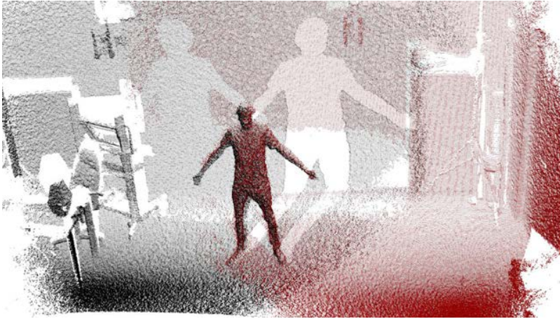
Figure 7.12: Point cloud fusion with two Kinect v2 cameras. Human depth information becomes more dense and concealed structures can be captured using multi-sensor arrangements
