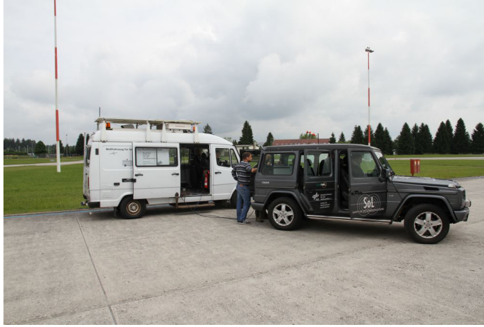
Figure 3.1. TX vehicle on the right and RX vehicle on the left are connected via cable, while the measurement crew conducts the calibration procedure to synchronize the atomic clocks.
