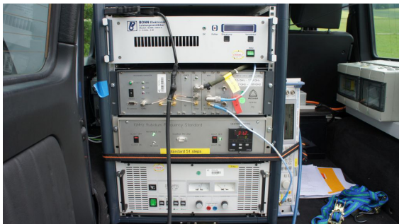
(a) From top to bottom: amplifier, PTS, atomic clock, 24 V power supply, and signal generator in the TX vehicle.
