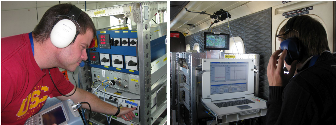
(a) From top to bottom: power box, PTS and amplifier installed in rack 2 of the TX aircraft.
