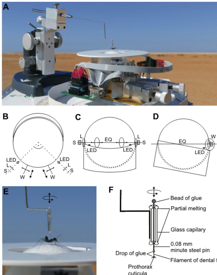
**Fig. 1. Closed-loop system: experimental setup and animal tethering.** (A) *Cataglyphis fortis* on the closed-loop treadmill with a styrofoam sphere of 5 cm diameter in the desert of Tunisia (complete overview).
