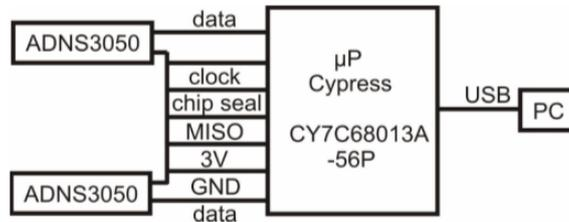
**Fig. S4: Sensor- $\mu$ P connections**
