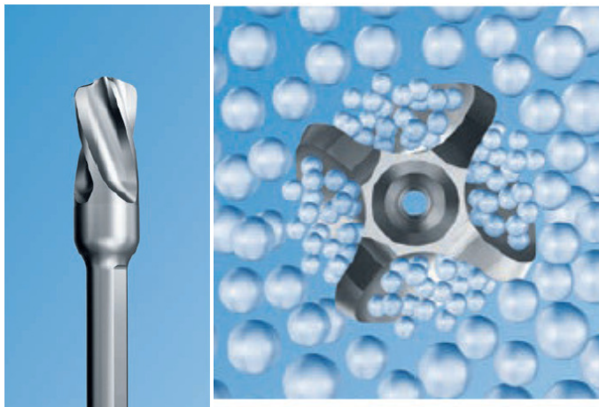
Fig.6: The design of the screw tip was changed from a threaded and cutting to a winded and volumetric impacting geometry, allowing volumetric impact of the surrounding bone mass (shown as bubbles). With kind permission of DePuySynthes.
