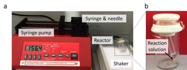
Figure S3 Home-designed device for the ATRP reaction. a , The device was composed by a syringe pump, syringe, needle, reactor ( b ), and shaker. Inside the argon filled reactor, a small vial is standing, in which the reaction solution was contained.
