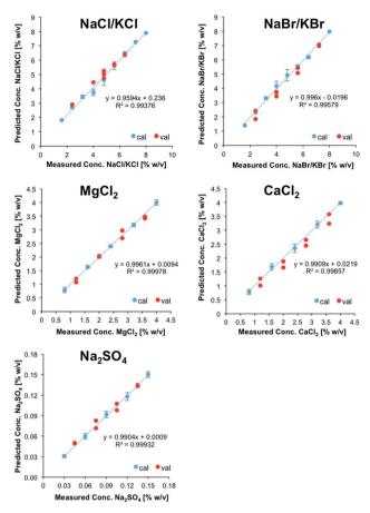
Fig. 2 Linear calibration functions for ion pairs derived from IR-ATR spectra. NaCl and KCl, as well as NaBr and KBr were treated as sum parameters.
