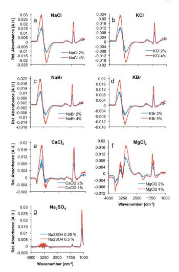
Fig. 1 Difference spectra of the salts investigated within the present study. (a) NaCl, (b) KCl, (c) NaBr, (d) KBr, (e)  $CaCl_2$ , (f) MgCl<sub>2</sub>, and (g) Na<sub>2</sub>SO<sub>4</sub>, each at two different concentrations. (a) and (b) as well as (c) and (d) were treated as sum parameters in the following analysis. All spectra were collected at a spectral resolution of 1 cm<sup>-1</sup> averaging 100 scans.
