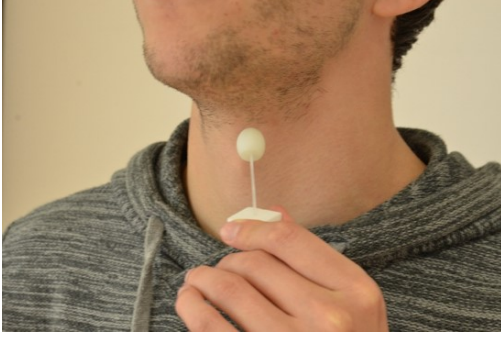
Fig. 3. Flexible positioning of the dielectric lens antenna at the throat for the vibration measurement.
