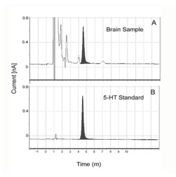
Figure 9. HPLC chromatograms (A/D Instruments Inc.; PowerChrom version 2.2.4) showing the peaks contained in a brain sample (A) compared with a serotonin (5-HT) external standard (B). (also see 2.3.8 for additional external standards tried).
