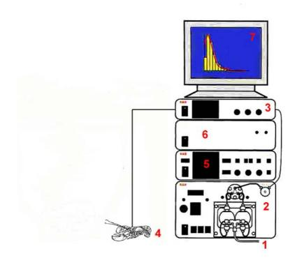
Figure 8. HPLC set-up showing the devices involved to read the analyte. (1) mobile phase enters the system via the pumps (2) and is pumped to the column (3). Here the sample (4) is injected onto the column and reads according to the detector settings (5) and via an A/D converter (6) on the computer (7).
