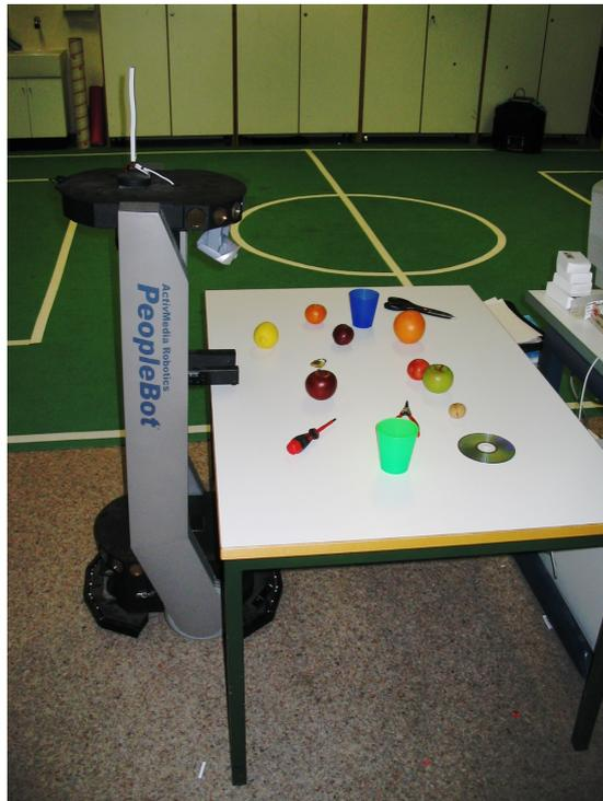
**Figure 9.2:** *MirrorBot test scenario. In the test scenario the robot is situated in front of a table. Different objects are lying on this table. The robot has to grasp or point to specified objects.*
