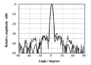
**Fig. 5:** Radiation diagrams of the V-band folded reflector antenna at 61.2 GHz. (Solid line: theory, dotted line: measurement E-plane).
