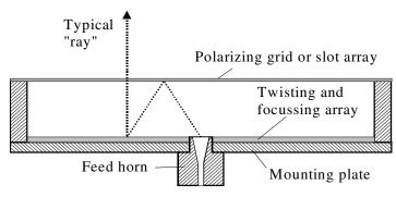
Fig. 2: Basic principle of the folded reflector antenna.
