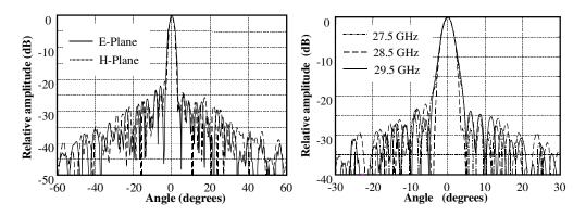
**Fig. 4:** Radiation diagrams of the Ka-band folded reflector antenna. (Left side: E- and H-plane at 28.5 GHz. Right side: E-plane at 27.5, 28.5, and 29.5 GHz).
