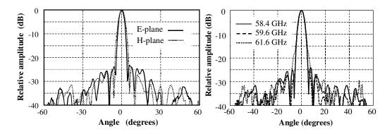
**Fig. 5:** Radiation diagrams of the V-band folded reflector antenna. (Left side: E- and H-plane at 58.4 GHz. Right side: H-plane at 58.4, 59.6, and 61.6 GHz. Reflectarray and grid: Duroid material of 0.254 mm and 1.58 mm thickness, respectively).
