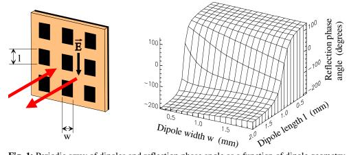
**Fig. 1:** Periodic array of dipoles and reflection phase angle as a function of dipole geometry (Substrate thickness 0.254 mm, dielectric constant 2.22, dipole distances 2.2 mm × 2.2 mm, f = 76.5 GHz).
