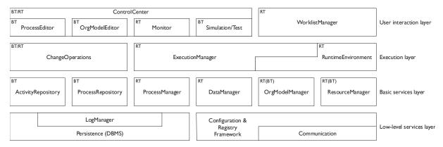
Figure 13: Basic Architecture of ADEPT2 (BT: Buildtime; RT: Runtime)
