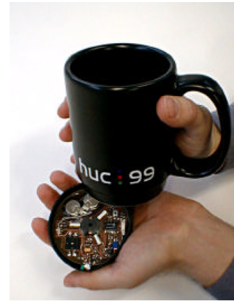
Figure 3. The Mediacup - An ordinary coffee cup equipped with sensor technology [1]
