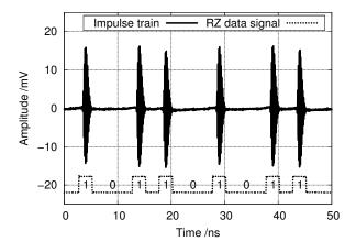
Fig. 5. Measured time domain output waveform of an 200 MBit/s OOK modulated impulse train.
