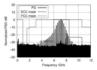
Fig. 4. Measured normalised spectral power density in a 1 MHz measurement bandwidth of the impulse generator at a repetition rate of 200 MHz compared to the FCC and the ECC spectral masks.
