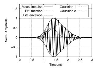
Fig. 7. Comparison of normalised measured and fitted time domain output waveform, including the envelope functions and the two Gaussian functions used to build the envelope function.
