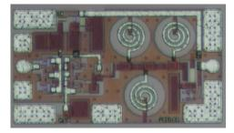
Fig. 6. Micrograph of the monolithic impulse generator circuit. The IC has a size of  $480 \times 880 \,\mu\text{m}^2$ .
