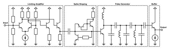
Fig. 2. Simplified circuit schematic of the impulse generator. Only part of the bias arrangement is shown here.
