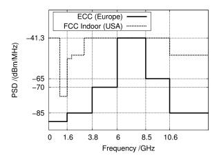
Fig. 1. The European UWB mask compared to the FCC indoor mask.
