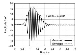
Fig. 3. Measured time domain output waveform of the impulse generator.
