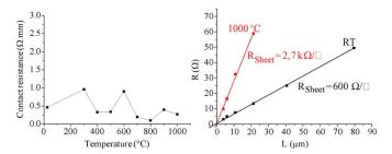
Fig. 4. (Left) Change of contact resistance with operating temperature. (Right) Extrapolation of planar contact resistance and sheet resistance from TLM measurements at measurement temperatures of RT and  $1000\,^{\circ}$ C.
