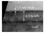
Fig. 5. TEM cross section of lattice-matched InAlN/GaN heterostructure with 10-nm barrier thickness. (Left) Heterostructure before oxidation. (Right) Heterostructure after oxidation at  $800\,^{\circ}\text{C}$  in  $O_2$  for 4 min [46].
