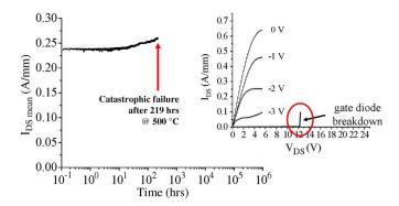
Fig. 8. Failure cycle of AlGaN/GaN HEMT device as described in the text. Operation conditions:  $R_L=500~\Omega,~V_{\rm DS}=20~\rm V,~V_{\rm GS}=-3.6$ –0 V,  $f_{\rm in}=1~\rm MHz$ , and temperature stepping from 300 °C to 500 °C.
