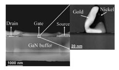
Fig. 13. HAADF STEM image of cross section of the gate, source/drain region after 30 min annealing at 800  $^{\circ}\text{C}.$
