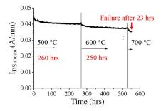
Fig. 10. Test cycles of InAlN/GaN HEMT up to failure. Failure occurred after 23 h at 700  $^{\circ}\mathrm{C}.$
