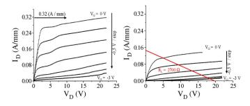
Fig. 15. Output characteristics of the InAlN/GaN HEMT device discussed in Fig. 14. (Left) Device at RT. Kink in the output characteristics is related to charge injection into the buffer, leading to a shift in the internal gate voltage. (Right) Device with  $800\,^{\circ}\text{C}$  load line selected for  $800\,^{\circ}\text{C}$  operation.
