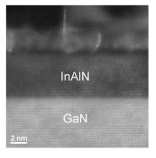
Fig. 2. HAADF STEM image of cross section of Ti/Al/Ni/Au contact annealed at  $800\,^{\circ}\text{C}$  on InAlN/GaN heterostructure.
