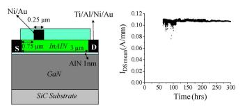
Fig. 9. (Left) Device cross section of the InAlN/GaN HEMTs. First- and second-generation devices differ only in the ohmic and gate contact metallization schemes. (Right) 500  $^{\circ}$ C test step of a typical InAlN/GaN device with lattice-matched barrier layer.
