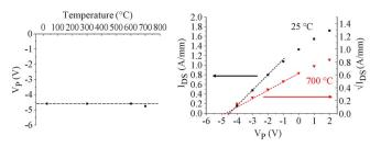
Fig. 11. (Left) Change of extracted pinchoff voltage (see right) at operating temperature of  $L_g=0.25~\mu \rm m$  FET. (Right) Extraction of pinchoff voltage at the onset of saturation: At 25 °C from linear transfer characteristic (highmobility short-channel case and at 700 °C extraction from the square root plot of the transfer characteristics (low-mobility long-channel case).
