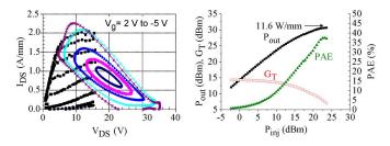
Fig. 6. Large-signal 4-GHz power performance of InAlN/GaN MISHEMT structure, including hard input overdrive conditions. Device data:  $t_{\rm InAlN}=10$  nm,  $T_{\rm oxide}=1.5$  nm,  $L_G=0.25~\mu{\rm m}$ , and  $W_G=2^*50~\mu{\rm m}$ . In part after [48].
