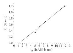
Fig. 3. Dependence of planar contact resistance as function of InAIN barrier thickness [27].
