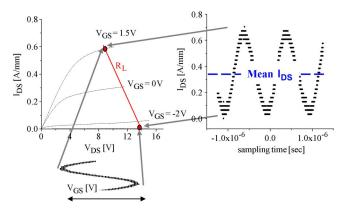
Fig. 7. Test arrangement of temperature stepping experiment. Input signal 1 MHz; bias point and amplitude adjusted as shown. Output terminated by  $R_L$ . Output waveform recorded every  $60~\rm s.$
