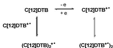
Scheme 3.25: Proposed dimerization between charged and uncharged macrocycles.
