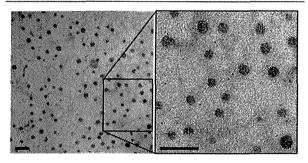
Figure 1. Transmission electron micrograph of polyfluorene nanoparticles prepared by miniemulsion polymerization (0.06 wt %=2 equiv of NaOH and 1 wt % aqueous SDS). The scale bars correspond to 100 nm.
