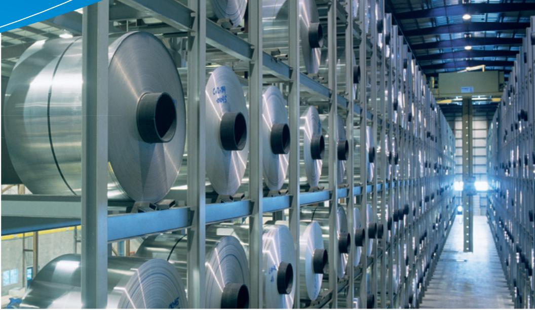
Storage unit in aluminium plant with automated storage and retrieval
