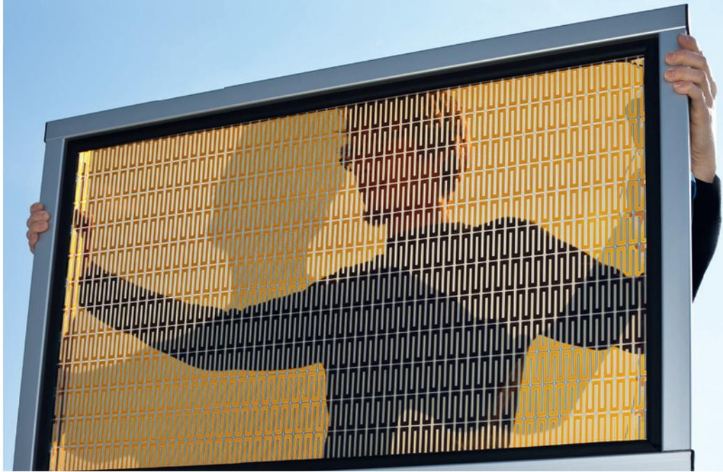
A prototype of a screenprinted dye-sensitised solar panel produced by Fraunhofer ISE
