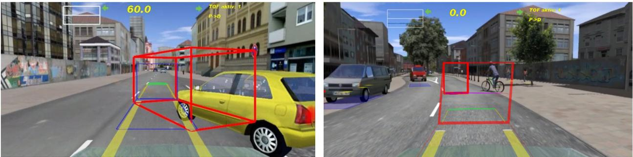
**Figure 2.2** Predictive display visualizing the path of the ego vehicle as well as the actual front position of the ego vehicle and other traffic participants (source: [9] © 2016 IEEE).
