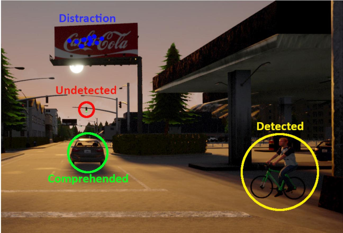
**Figure 4.10** Visualization of the circular ROIs representing the optimal SEs and their perception level. The *undetected* SE is visualized in red, the *detected* SE in yellow, and the *comprehended* SE in green. The accumulation of gaze points in blue on a non-ROI area will be considered by the distraction penalty. Adopted from [22] © 2020 IEEE.
