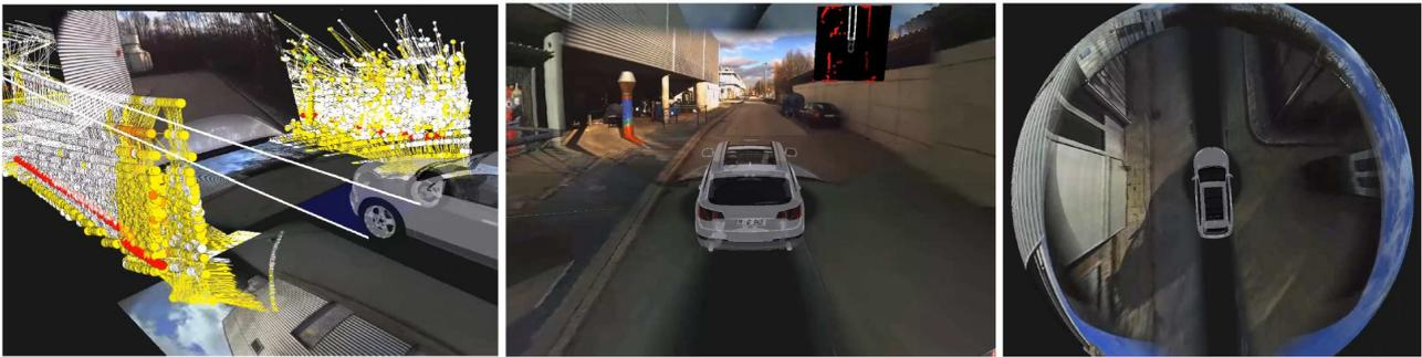
**Figure 2.3** Three visualization types supported by the ToD interface. A LiDAR point cloud augmented with camera data is shown on the left. In the middle, all fisheye cameras, a front camera, and LiDAR data are combined in to a single representation. The right view shows a birds-eye view based on the fisheye cameras (source: [55] © 2019 IEEE).
