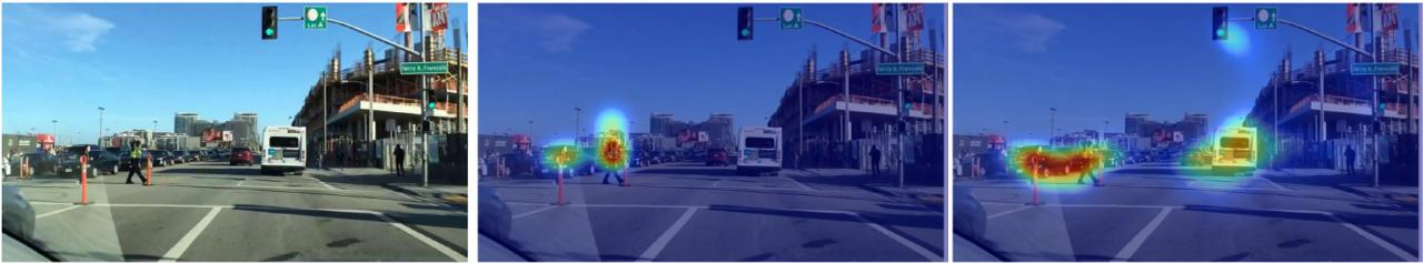
Figure 2.5 Raw image and gaze heatmap accumulated from multiple drivers (source: [95]).
