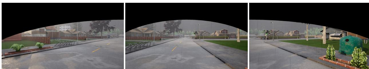
**Figure 5.3** Three camera views with ROI masks. Left: A left-facing camera view. Center: A front-facing camera view. Right: A right-facing camera view.
