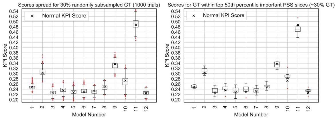
**FIGURE 10** Comparison of KPI scores from NPRS against top 50<sup>th</sup> percentile important PSS
