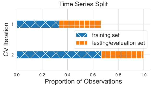
FIGURE 4. Time series split cross-validation (CV) train and test sets.
