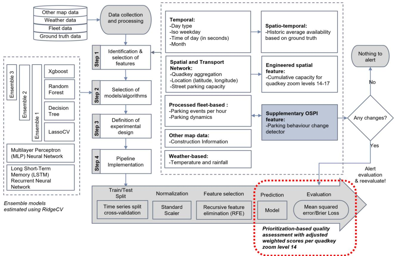
FIGURE 5. Development methodology workflow for an OSPI system.
