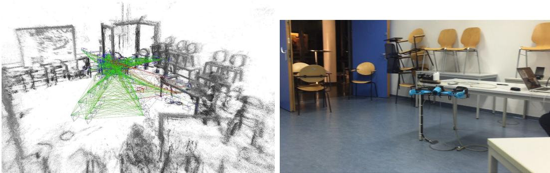
Figure 1.2: Example of how a quadcopter can autonomously explore an unknown environment, utilizing a visual SLAM system. This work was published in [1] and is based on the Bachelor’s thesis [57] of Lukas von Stumberg.
