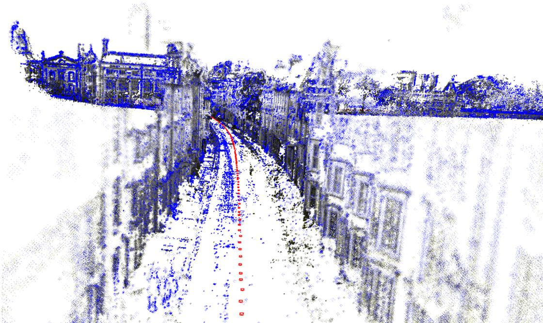
Figure 2.3: Relocalization demo on the Oxford RobotCar dataset. We relocalize sequences with different weather conditions (sunny and snowy in this example) and overlay the pointclouds using the estimated transformations. The pointclouds align very well, showing that the relocalization is accurate.
