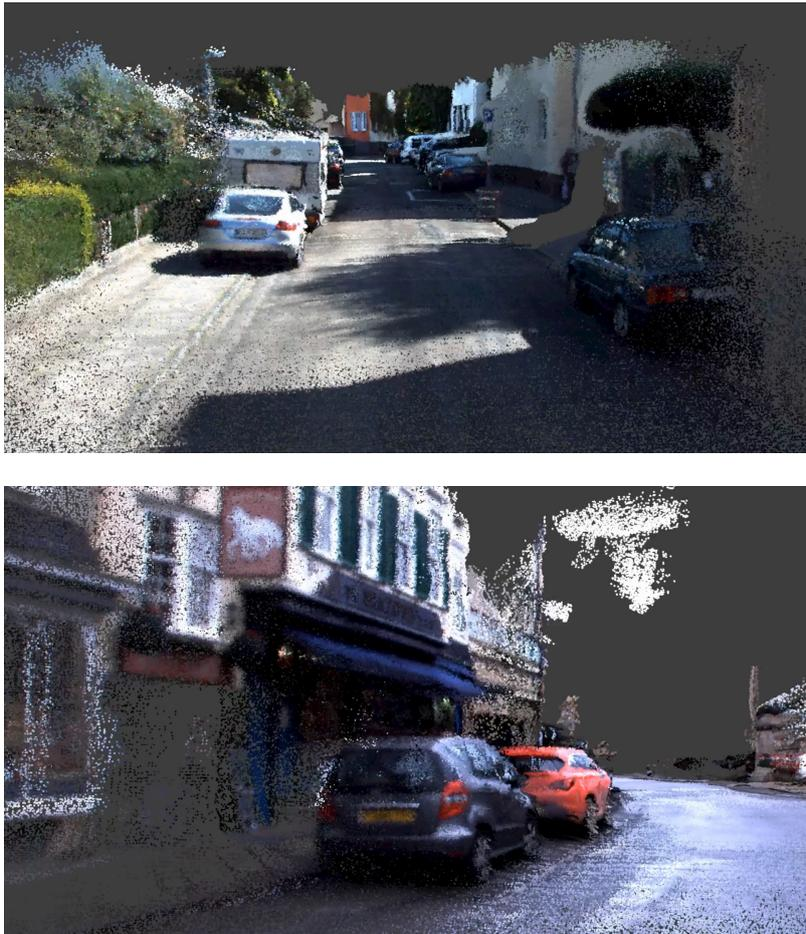
Figure 1.3: Accurate poses from SLAM can also benefit downstream computer vision tasks. MonoRec [3], a work led by Felix Wimbauer, achieves accurate 3D reconstruction using a cost volume, relying on accurate poses from visual odometry.
