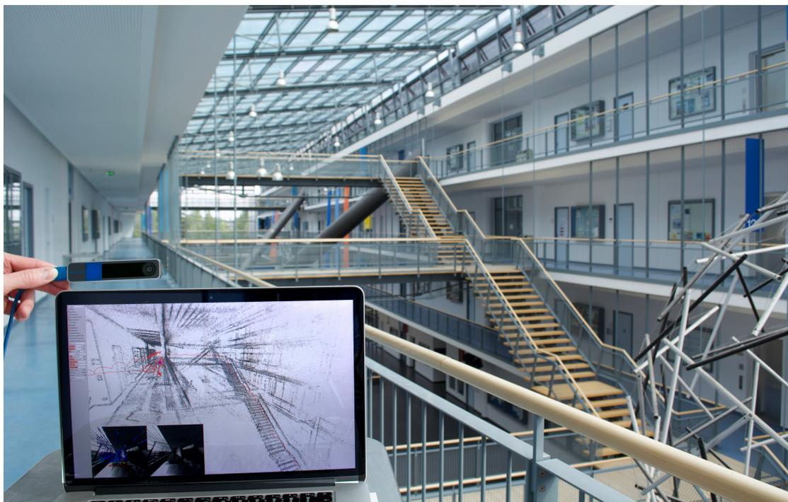
Figure 1.1: DM-VIO (Chapter 4) running live on a laptop, connected to a monocular camera with integrated IMU. It reconstructs the trajectory and 3D environment (pointcloud on the laptop) with remarkable accuracy in real-time. The source-code for this live demo has been released, see Appendix B.
