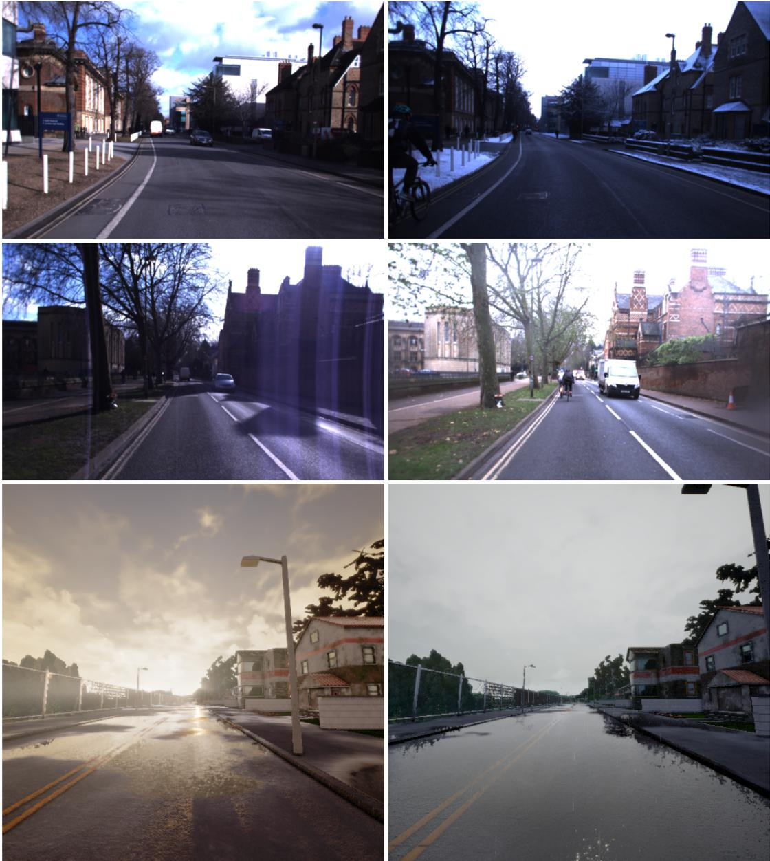
Figure 6.6: Example image pairs from the relocalization tracking benchmark which have been successfully relocalized by LM-Reloc (with an accuracy of better than 10 cm). Top row: Oxford sunny against snowy condition, middle row: Oxford sunny against rainy condition, bottom row: CARLA benchmark.
