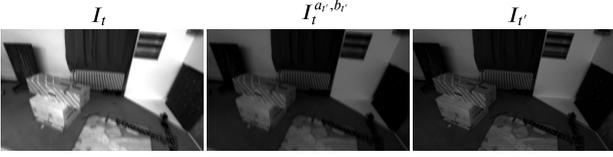
Figure 3: Examples of affine brightness transformation on EuRoC MAV [5]. Originally the source image ( $I_{t'}$ ) and the target image ( $I_t$ ) show different brightness. With the predicted parameters  $a, b$ , the transformed target images  $I_t^{a,b}$  have similar brightness as the source images, which facilitates the self-supervised training based on the brightness constancy assumption.
