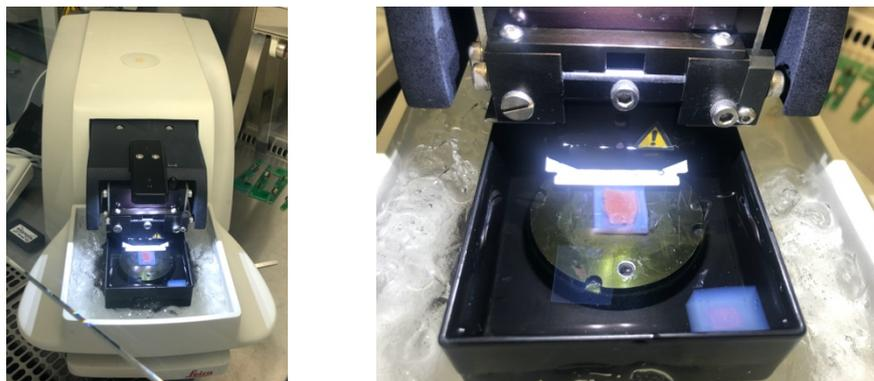
**Figure 9. Vibratome in use.** The prepared 4 % agarose block that contained the embedded LV NHP heart tissue was positioned in the cooling bath at 4 °C, where it was surrounded by ice. The slicing process was performed by the Vibratome, and the LV NHP heart slices were processed further immediately after cutting.
