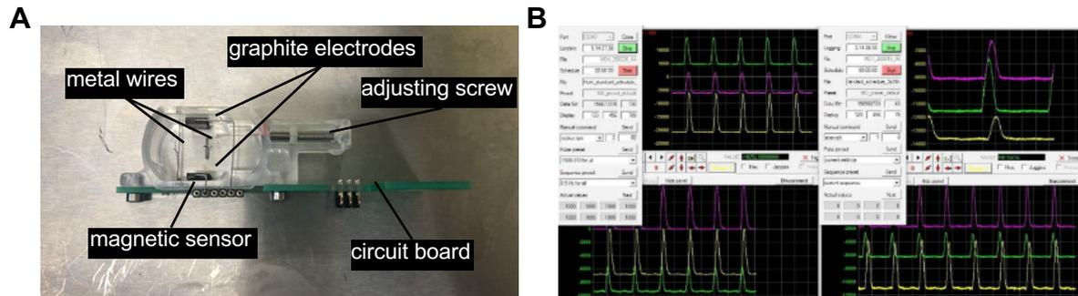
**Figure 12. Hardware and software of the culture platform system. A** Top view of BMCC. **B** Desktop view of programme MyoDish in use. Individual contractile traces can be observed.
