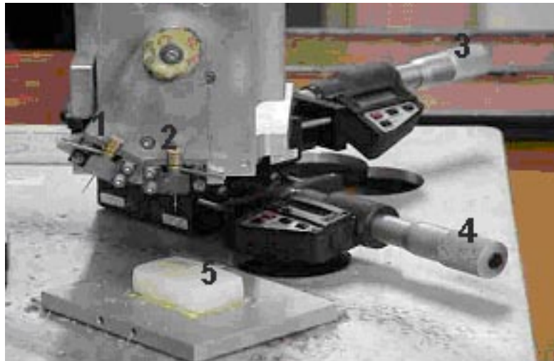
Figure 2. Tissue arrayer and its working principle. Adjusting front-back alignment of a punch with the setscrews (3 and 4) located in front of the arrayer. Samples from the donor block are aspirated and arrayed into a new recipient paraffin block (5). 1 is a punch for making a hole in the recipient block, and 2 is a punch for aspirating, transferring and depositing samples.
