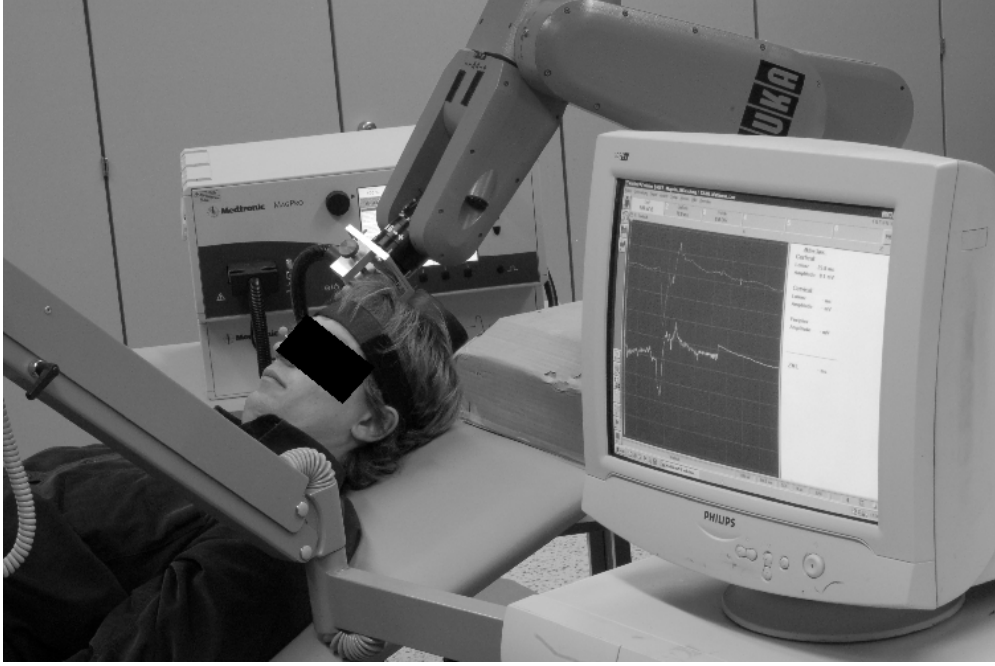
Figure 5.1.: Experimental setup for motor cortex mapping. The head is tracked using a marker attached to the head. Motor evoked potentials (displayed on the computer screen in the foreground) are recorded from the right abductor pollicis brevis muscle (a muscle that moves the thumb, APB) and related to the coil position at the head.
