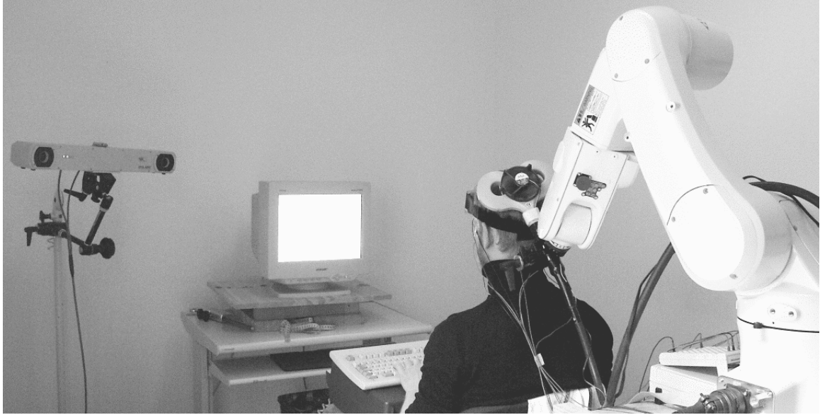
Figure 5.5.: Setup of the RSVP experiment. The robot is positioned over electrode position P3 (here) or P4 and kept in place during the experiment using motion compensation. Electrodes at P7 and P8 measure EEG responses in the visual cortex, electrodes on the face measure the eye movements to correct for EOG (electrooculographic) artefacts in the EEG. The subject follows the display of letters on the screen and types on the keyboard the letter which was not black and number appearing afterwards. Head motions are tracked using the headband the subject wears and the Polaris tracking camera on the left.
