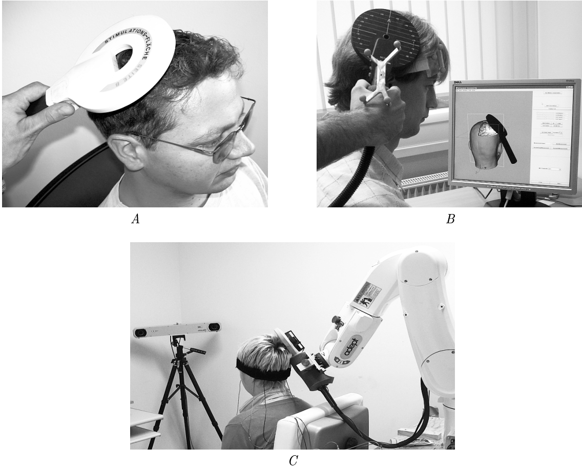
Figure 1.2.: Evolution of coil placement in TMS. A: Manual coil placement without guidance. B: Manual coil placement with support from image guidance. C: Coil placement by a robot, compensating for head movements e.g. during a TMS-EEG experiment.
