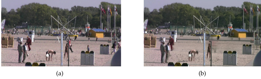
Figure 6.7: Example stillshot from “temporal foveation” experiment. (a) Original video frame. (b) Video frame after gaze-contingent temporal filtering; gaze position is indicated by the white marker at the left image border below the sail. The static background (low temporal frequencies) is unmodified, but moving objects are progressively filtered out with increasing distance from gaze (note that two walkers in the original frame have disappeared). The resolution falloff is described by the curve in Figure 6.6(b).
