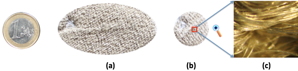
Fig. 5-12: The textile electrodes used for the Active Belt system. (a) A elliptical electrode, (b) a circular electrode and (c) a microscopic (40x) view of ELITEX ® threads.
