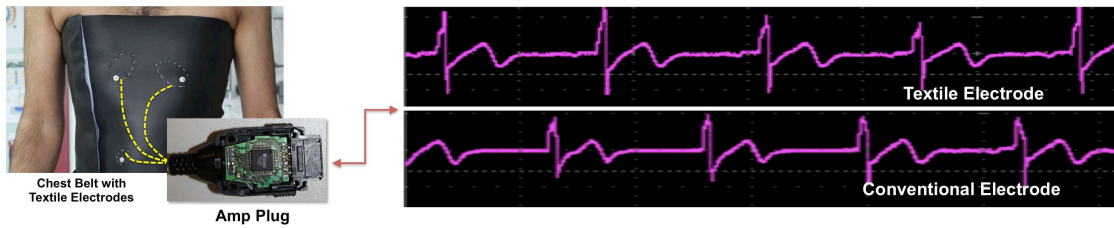
Fig. 5-25: ECG recorded by the Amp Plug.
