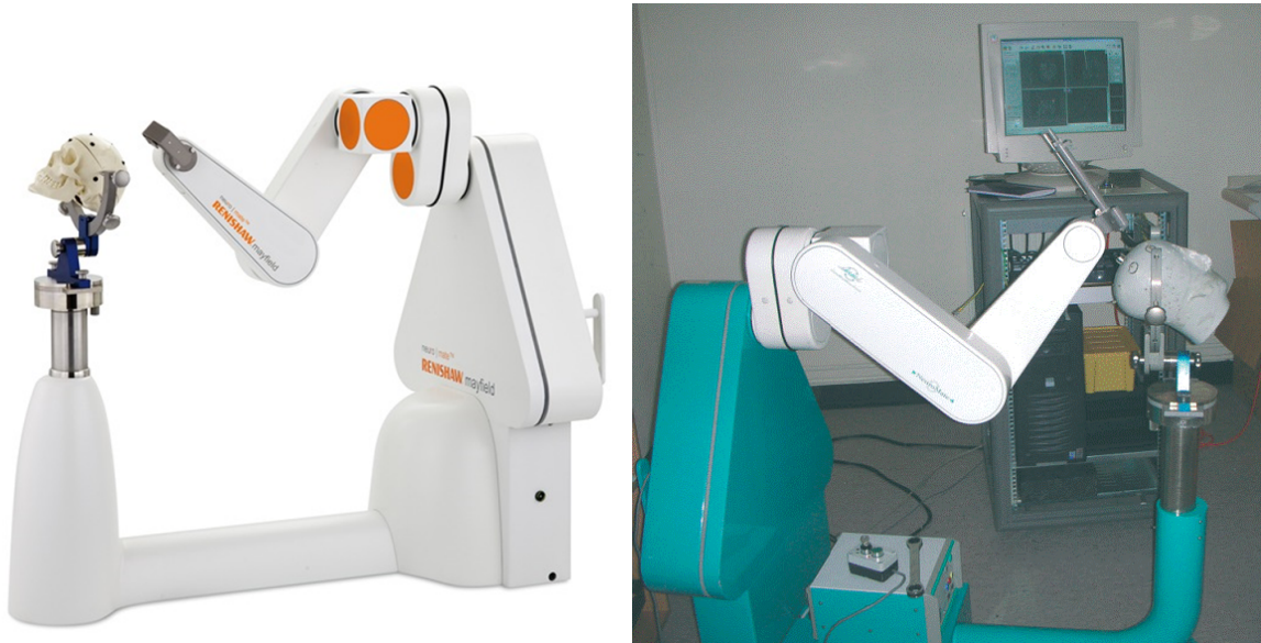
Figure 2.4: The CE/FDA approved neuromate system by Renishaw PLC, UK; Left: Currently distributed robot with phantom head attached to the head clamp. Right: previous version of the neuromate system with control unit in the background. Images courtesy of Renishaw GmbH.
