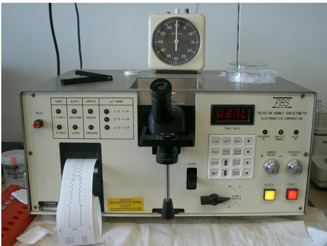
Abb. 12 Pulsating-Bubble-Surfactometer (PBS)
