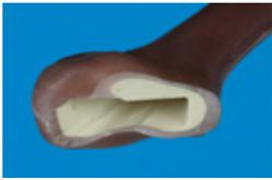
Fourth-generation bones model natural cortical bone using a mixture of short glass fibers and epoxy resin pressure injected around a foam core. Standard bone models are manufactured with a solid rigid polyurethane foam cancellous core material, unless cellular rigid polyurethane foam is specified. The mid-shaft area has an intermedullary canal.
