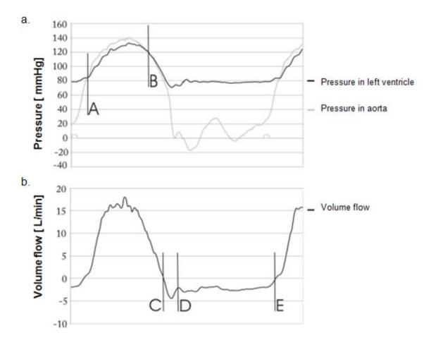
Fig. 7: Exemplary pressure and flow curves of one measured model in the study. a.: pressure curve. Equivalently, A=TVP mean (mmHg); B=TVP max (mmHg); b.: volume flow curve. C-D=V closure; D-E=V leakage.
