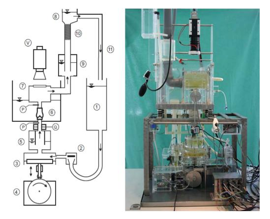
Fig. 5: Schematic depiction of hydrodynamic test circuit as a flow simulator [29] and finished model. 1.) atrial preload; 2.) mitral valve; 3.) pistons; 4.) electric power with control disk; 5.) ventricular compliance; 6.) testing space; 7.) deflection chamber with inspection glass; 8.) height variable liquid column; 9.) aortal compliance; 10.) peripheral resistance; 11.) return flow; P=pressure measurement; Q=volume measurement; V=video camera.
