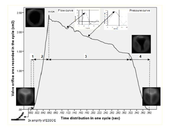
Fig.12: The graphics is depicted from the data assessed in a test sequence to elucidate the motion characteristics during the cardiac cycle. 1= early systolic slow valve opening episode; 2=late systolic rapid valve opening episode; 3= early systolic slow valve closing episode; 4= late systolic rapid valve closing episode. MVOA= maximal valve opening area
