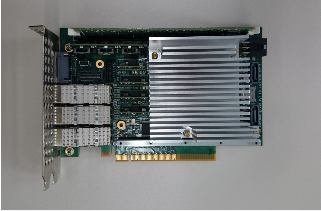
Figure 2.11 – FPGA board DNPCIe_10G_HXT_LL [100] used in this work.
