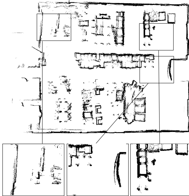
(a) Initial result obtained based on pose graph SLAM. Some structures appear multiple times on the map. Fine contours are not correctly mapped and seem to blur around objects.
