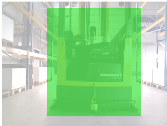
Figure 5.6.: Illustration of a region of interest (ROI) being detected using the depth image data and projected into the RGB camera's coordinate frame. The image content inside the ROI is passed to the feature extraction module.
