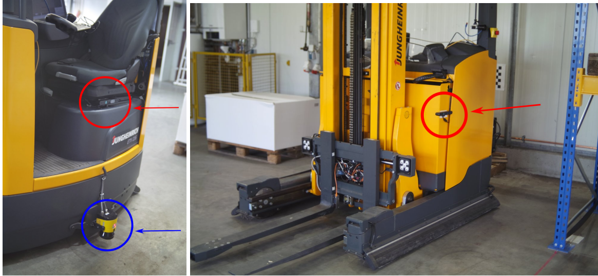
(a) Front RGB-D camera (red) and laser range finder (blue).
