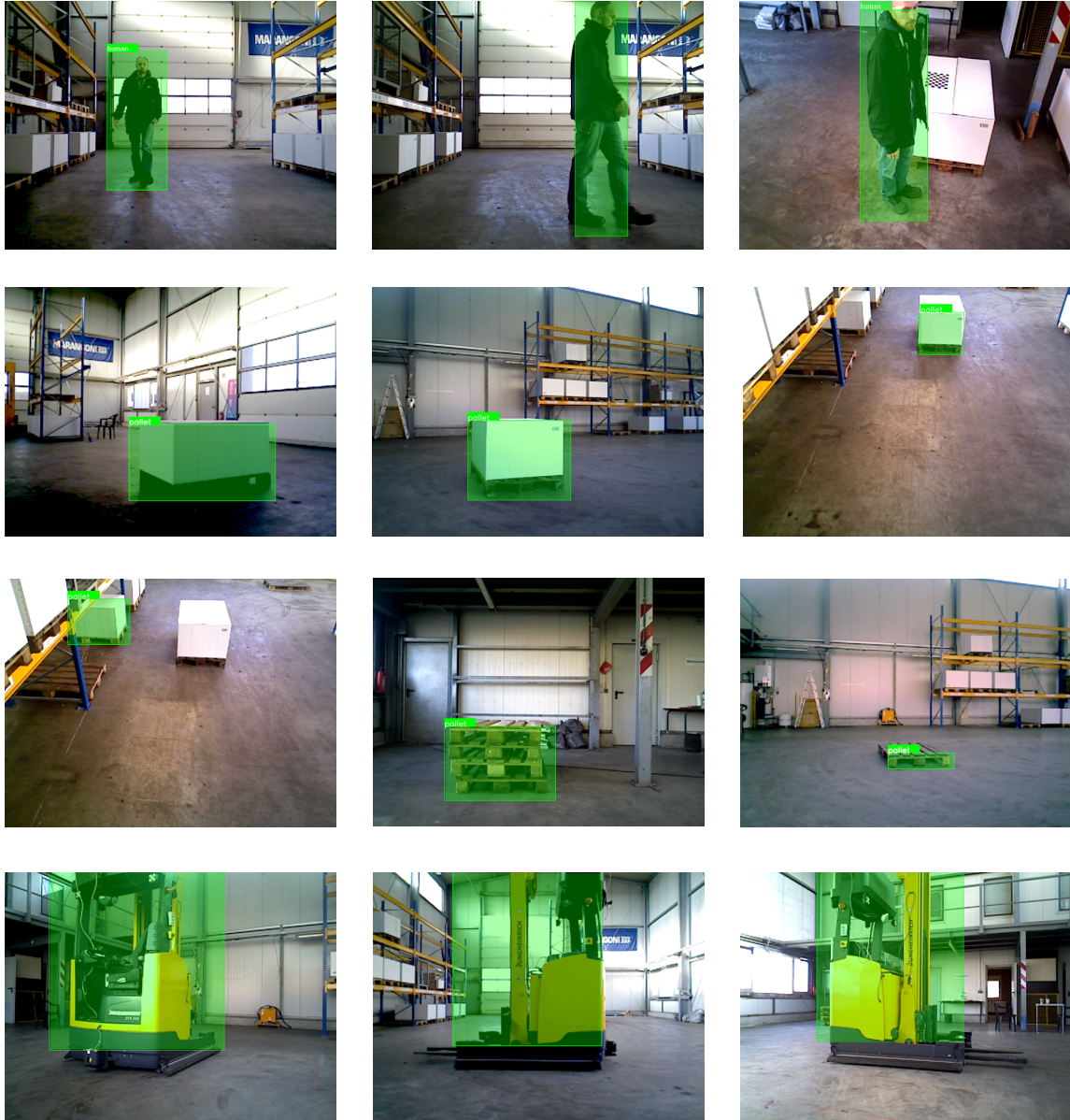
Figure 5.12.: Results obtained on the validation dataset captured in a warehouse environment. Our system is able to detect and recognize objects of the classes: forklifts , humans and palletized goods under varying poses and illumination conditions.
