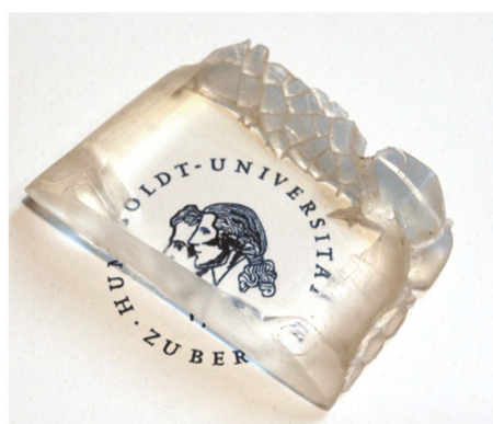
Fig. 21 Photograph of a representative composite sample with 10 wt% \text{MgF}_2 in a PolyHEMA matrix as bulk material (left) and refractive indices of thin film coatings based on magnesium and aluminium fluoride with different filler contents in a matrix of Poly(1,4-BDDMA) determined by ellipsometry (right). Reproduced from ref. 56 with permission of The Royal Society of Chemistry.
