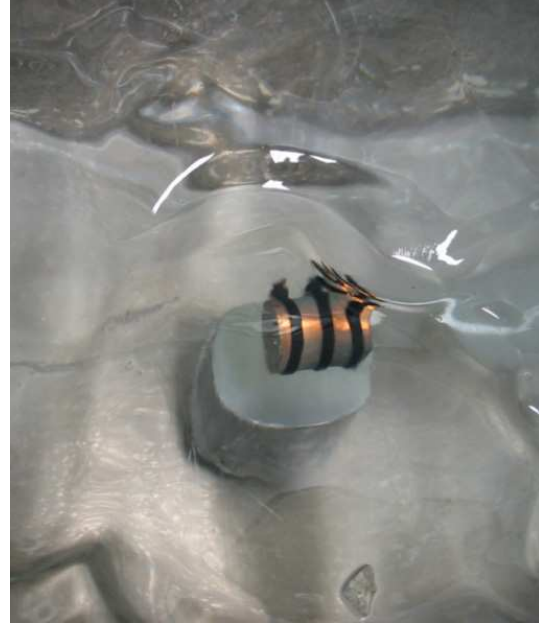
Figure 5.18: Epoxy sensor in a \approx 40 cm thick block of clear ice (from [Kri06]).
