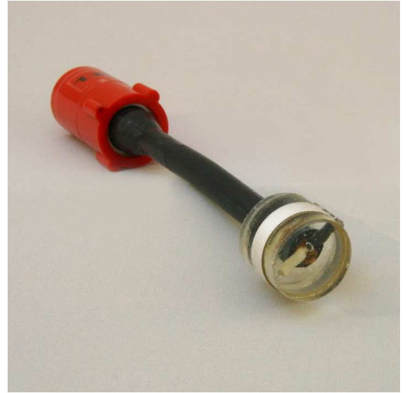
Figure 7.12: Ring-shaped ceramics cast in epoxy as used for the SPATS transmitters.
