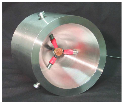
Figure 5.24: Directional acoustic emitter with parabolic reflector (from [Kri06]).
