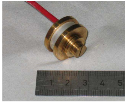
Figure 5.28: Transmitter with a ring-shaped PZT element sealed with o-rings.
