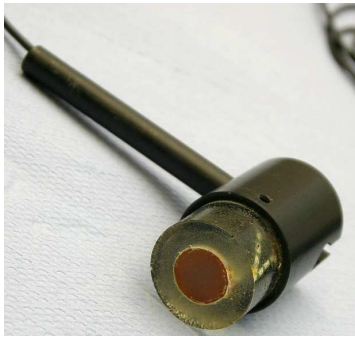
Figure 5.27: Transmitter with a cylindrical PZT element cast in epoxy.
