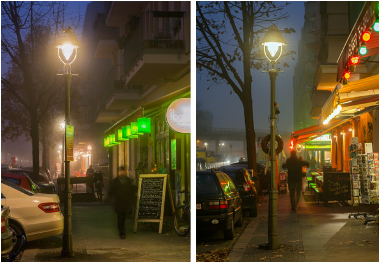
Figure 6-22: New LEDs (left) versus old gas lanterns (right) in Falckensteinstraße ©.
