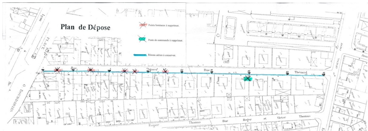
Figure 6-6: Five light points less for Rue Thénard and even larger pole distances (CC).
