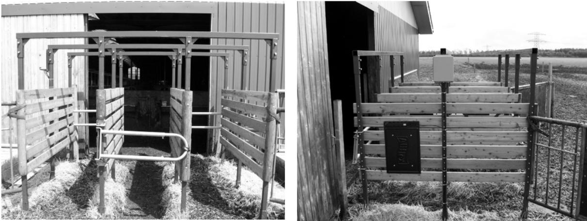
**Figure 3. Gates with RFID scanner**
